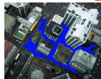
4. The base station estimates the plume boundary in real-time, predicts its future shape, and commands UAVs accordingly.
