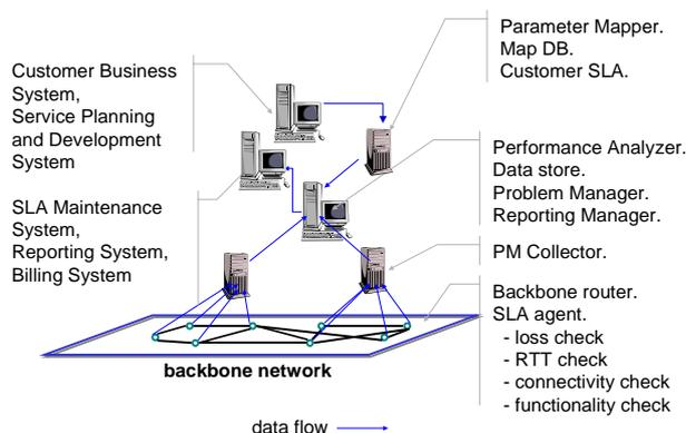
**Figure 8. Layered and Distributed SLA monitoring System in IP Backbone Network Service**
