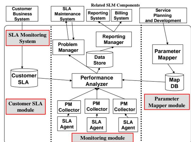
Figure 7. SLA Monitoring System Architecture
