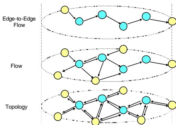
Figure 4. Mapping Relationships of Topology, Flow, and Edge-to-Edge Flow
