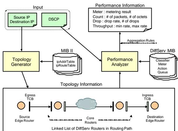
Figure 6. Construction of Edge-to-Edge DiffServ Flows
