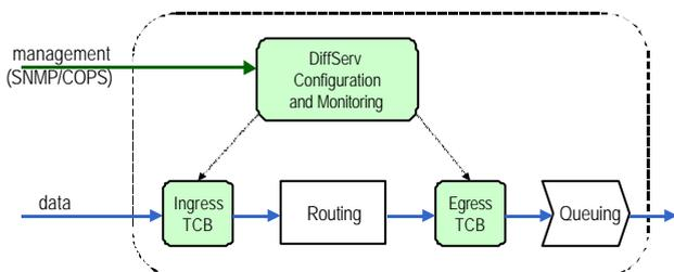
Figure 2. Conceptual Model of a DiffServ Router
